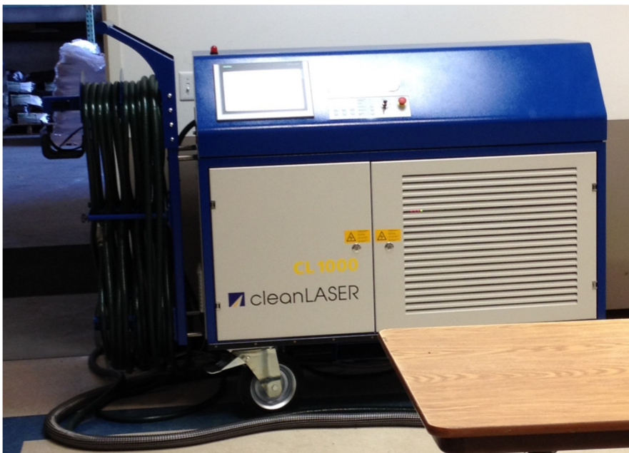
Figure 5: Filtration Cabinet - Located in Remote Area. Airborne contaminants are vacuumed from the LACR site to the HEPA filter, greatly reducing risk of exposure for the workers and the public
