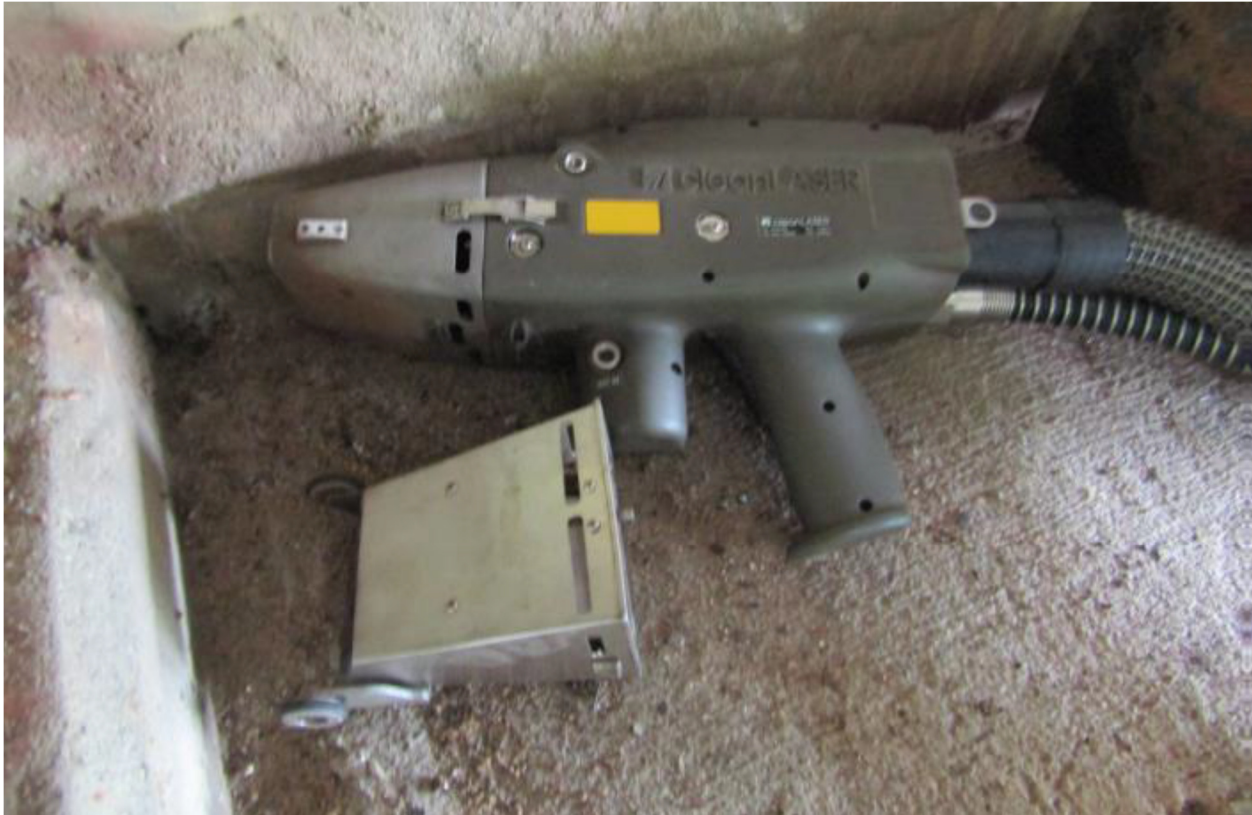
Figure 4: Photograph showing optic head and end-effector. Note the power feed and vacuum hose at the rear of the unit
